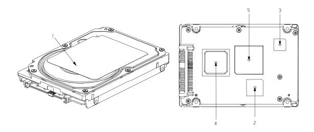
Figure 4.5 Surface temperature measurement points
